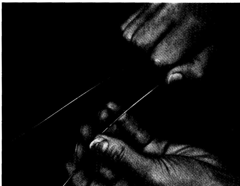
Fig. 98-8. Step 3. Straightening wire ends, making U shape of wire.
