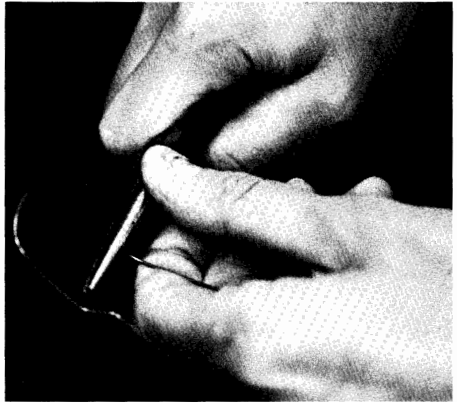
Fig. 98-10. Steps 6 and 7. Bending wire at 60-degree angles.
